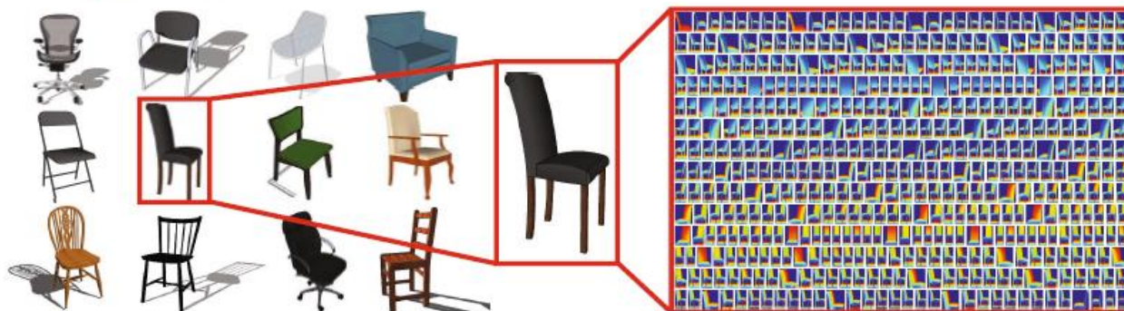
Fig. 2. Training procedure: We use a collection of CG models to train a 3D detector. For each CG model, we render it from hundreds of view angles to generate a pool of positive training data. For each rendering, we train an Exemplar-SVM model. And we ensemble all SVMs from renderings of CG chair models to build a 3D chair detector.
