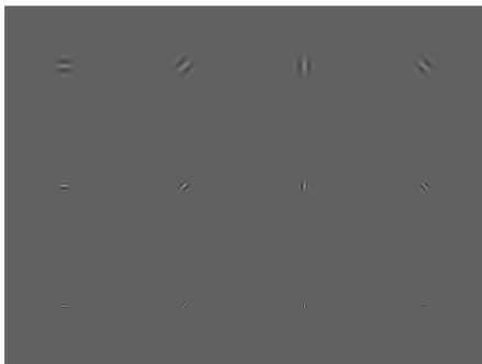
Figure 5.1: Filter responses of texture D3, produced by a bank of Gabor filters (3 scales and 4 orientations).
