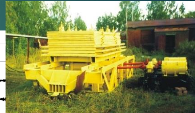
Seismic CV-40 vibrator
