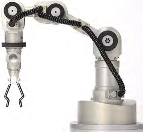
Рис. 5: Katana Robotic Arm
