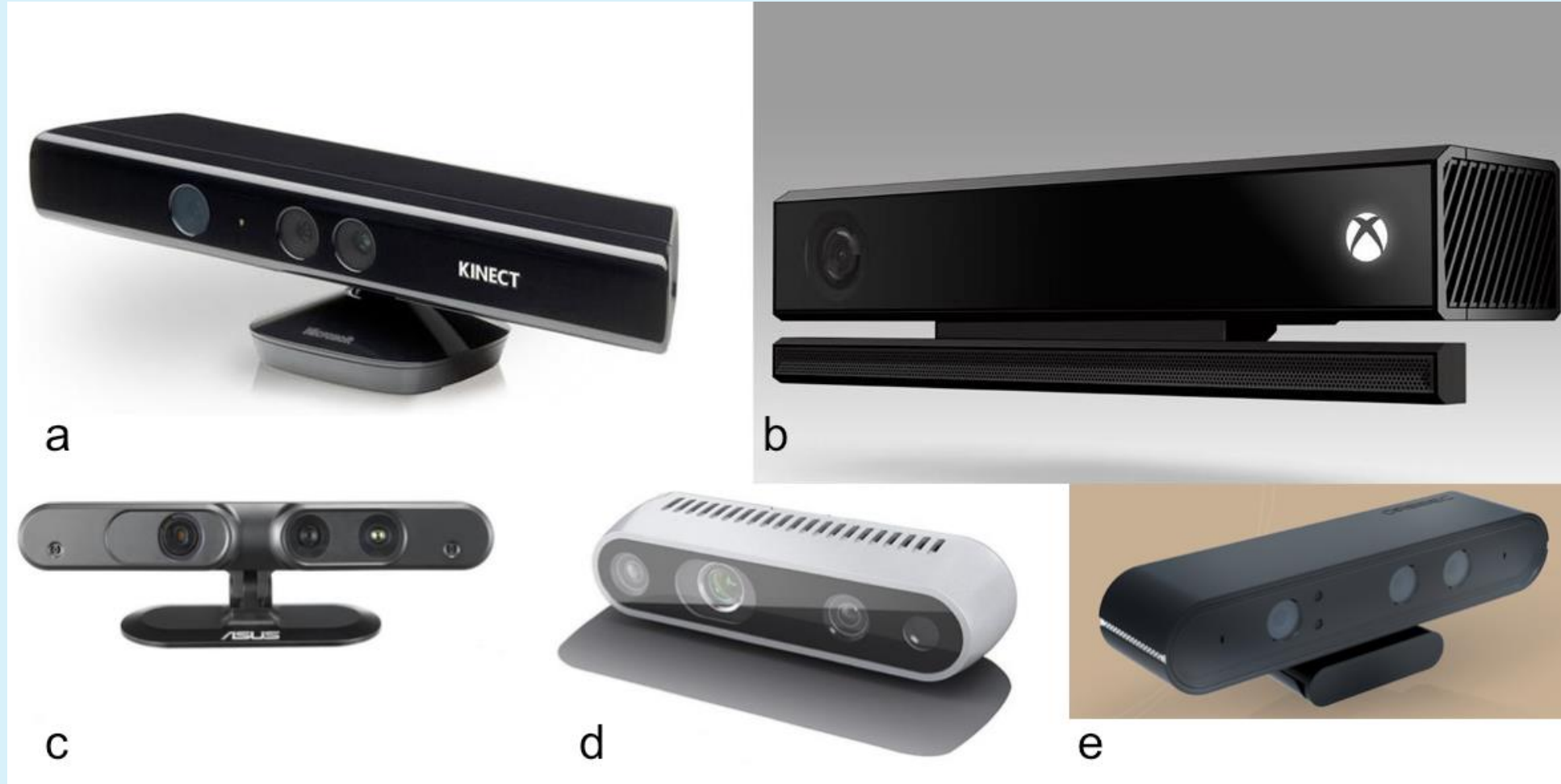
a - Microsoft Kinect v1, b - Microsoft Kinect v2, c - Asus Xtion PRO LIVE, d - Intel RealSense D435, e - Orbbec Astra pro
