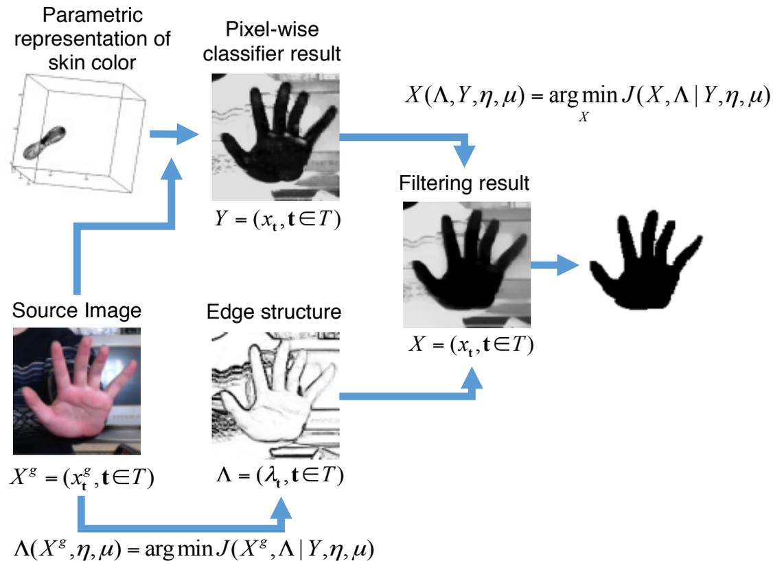
$$\begin{cases} (\hat{X}, \hat{\Lambda} | \eta, \mu) = \arg \min_{X, \Lambda} J(X, \Lambda | Y, \eta, \mu), \\ J(X, \Lambda | Y, \eta, \mu) = \sum_{t \in T} (y_t - x_t)^2 + \sum_{t', t'' \in T} \left\{ \frac{1}{\lambda_t} \left[ (x_{t'} - x_{t''})^2 + \frac{\eta}{\mu} \right] + \left(1 + \frac{1}{\mu}\right) \ln \lambda_t \right\}. \end{cases}$$
