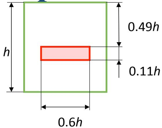
The parameters of training region inside the face rectangle are defined based on [2]. Particularly, just this area lies between the eyes and nose tip and is less deformable and free of beard, mustache, glasses, hair-dress, make-up.
