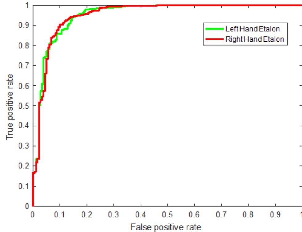
The quality of hands separation from the non-hand candidates is shown in the form of ROC-curve. This curve demonstrates the recognition true positive rate versus false positive rate along the increasing of comparison distance from the chosen etalon object. The AUC (area under the curve) for left hands (green curve) is equal 0.9535, and for the right hands (red curve) – 0.9531.
