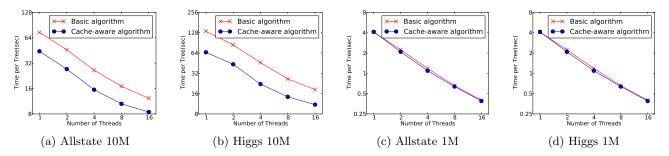
Figure 7: Impact of cache-aware prefetching in exact greedy algorithm. We find that the cache-miss effect impacts the performance on the large datasets (10 million instances). Using cache aware prefetching improves the performance by factor of two when the dataset is large.
