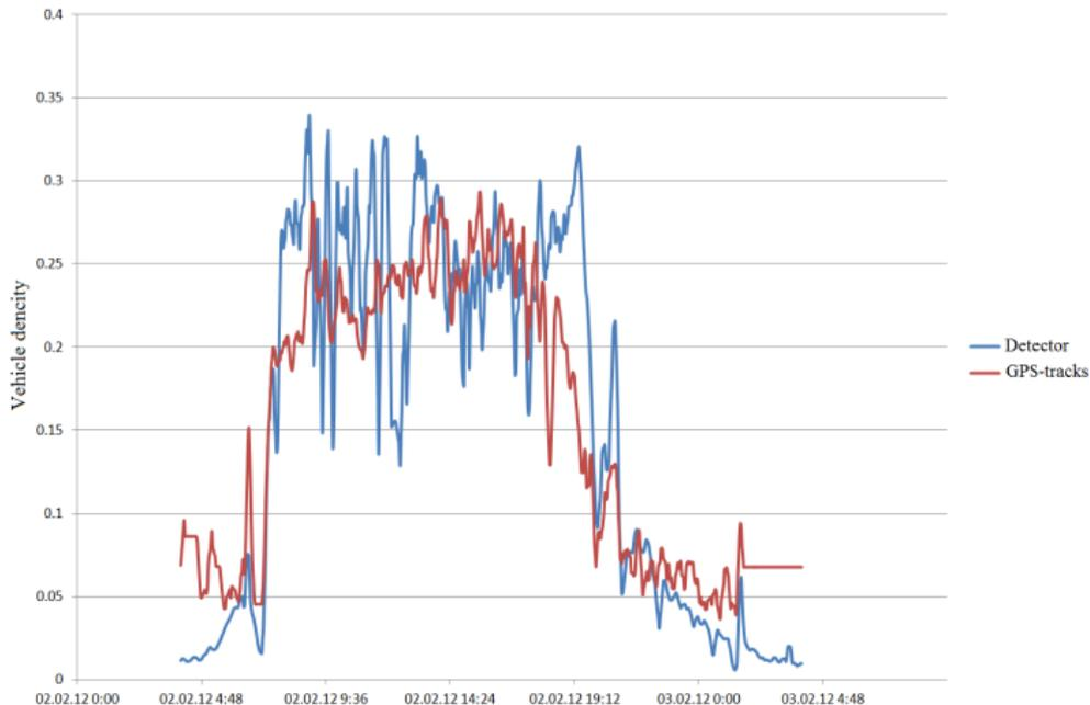
Figure: Vehicle density averaged on 10-minutes obtained after test<sub>1</sub> and ground truth.
