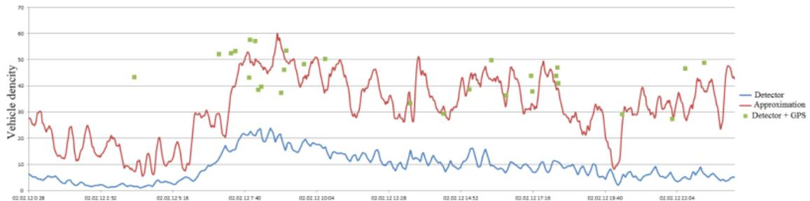
**Figure:** Blue line — data from traffic detector for one of the entrances, green dots — summary of data from data detector and GPS-tracks. Red line — recovered total number of entered vehicles  $N_{\text{estin}}$ .
