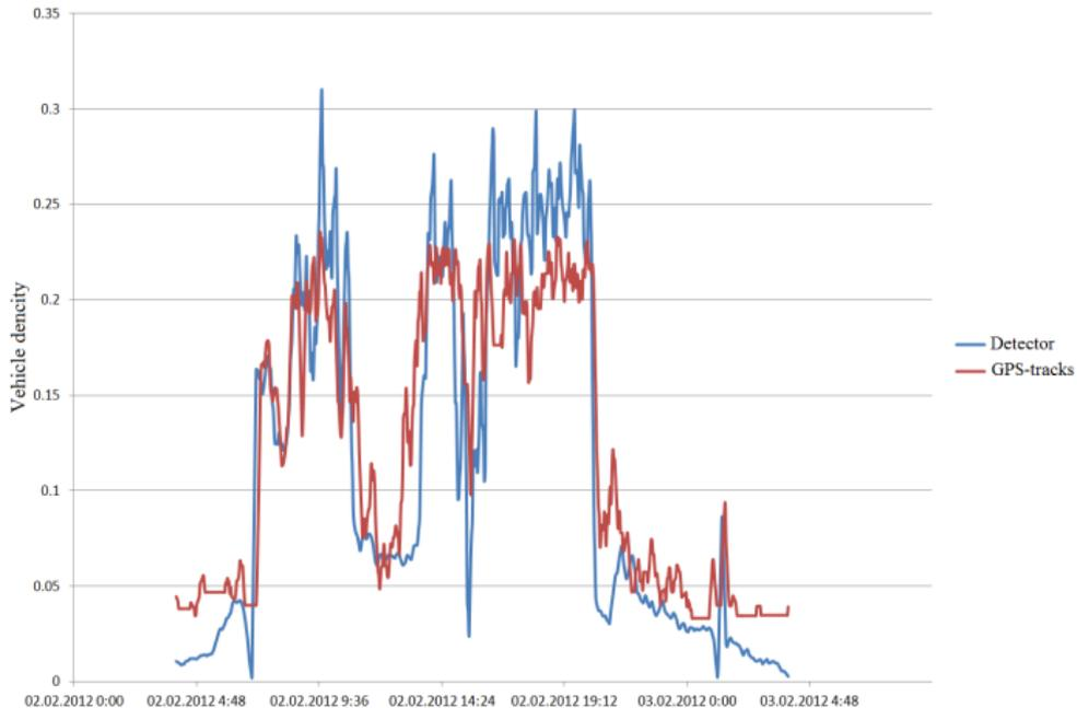
Figure: Vehicle density averaged on 10-minutes obtained after train and ground truth.
