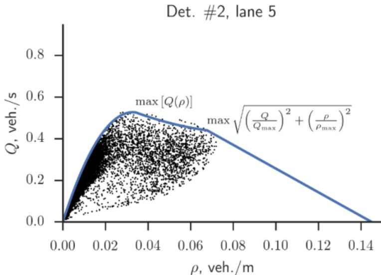
Figure: Fundamental diagram for Moscow Ring Road segment
