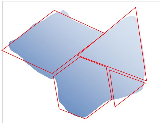
Fig.3. Covering  $\{L\}$  improved with unified representatives. Calculating membership in the class  $K_\lambda$  requires 3 convolutions instead of 16 ones.
